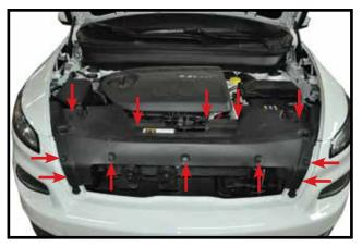
**1.** Open hood and remove twelve plastic push fasteners from top filler panel.
