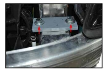
Place top support plate on each side of bumper and using 3/8" x 5" bolts, lock washers, and flat washers. Tighten the support brace till baseplate is pulled tight to bottom of bumper. NOTE: Use blue thread lock on all bolts.
