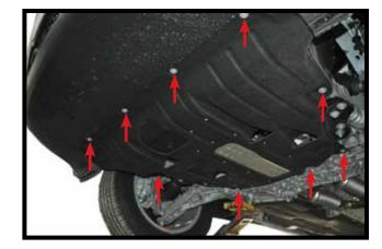
**5.** Remove nine bolts from skid panel and remove panel.
