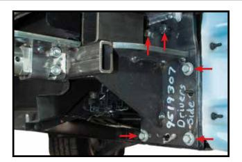
**10.** Tighten all bolts according to chart on front page in this order - bottom three, then lower bumper bolts, and then top support brace bolts.
