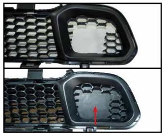
**11.** Trim lower grill as shown in picture. Trim as needed. **NOTE:** If equipped with active shutter system, trim solid plastic out behind grill webbing. Grill was taken out for clarity.
