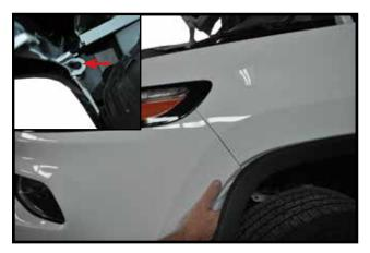
6. On each side remove one screw that attached the facia to the fender. Pull out and forward to remove facia. Unplug any wire connections that need to be unhooked to remove facia.
