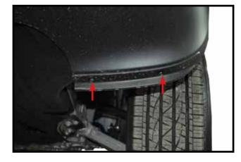
**4.** Drill out two aluminum rivets from front of each tire on the bottom of facia using 3/16" drill bit.
