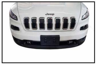
12. Replace facia and factory hardware in reverse order. Plug mount (item #12) may be installed if desired in convenience holes on either chain anchor or as desired. NOTE: Excess material may be trimmed from bracket.
